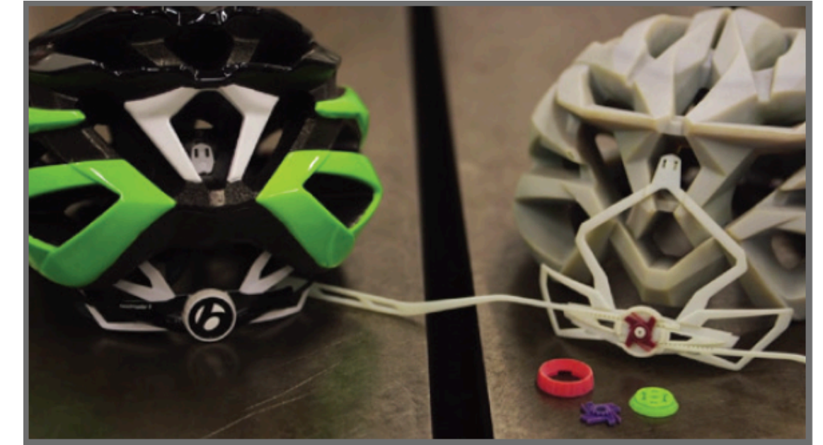
Trek's prototype development department uses multi-material 3D printing to achieve final-product realism.
