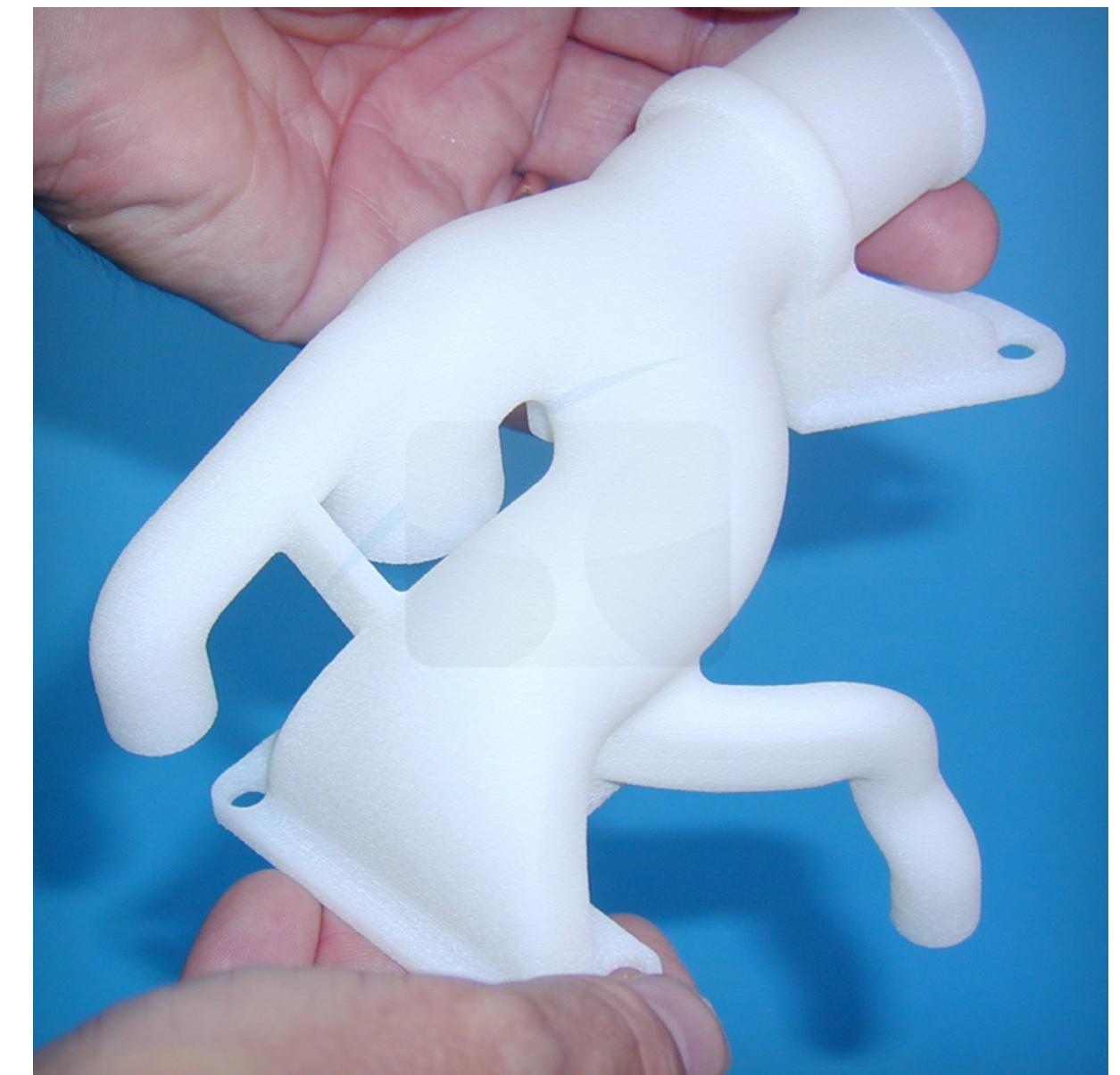
Trek's prototype development department uses multi-material 3D printing to achieve final-product realism.
