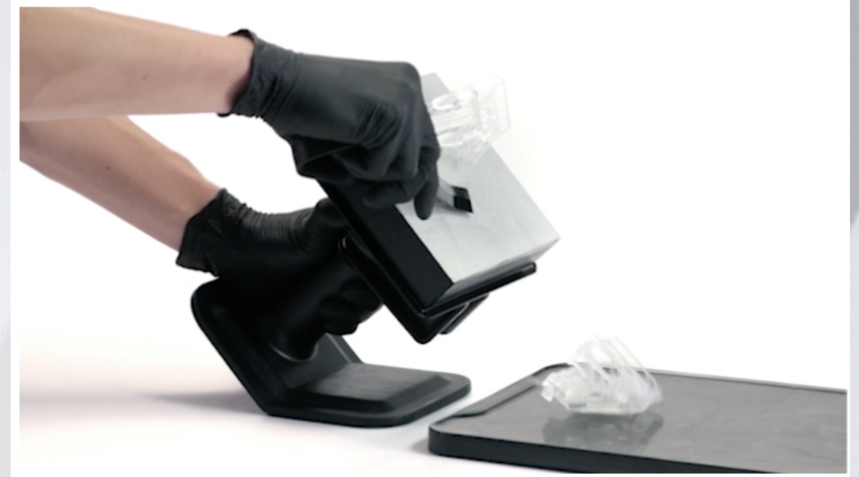
3. Use the removal tool to remove print
