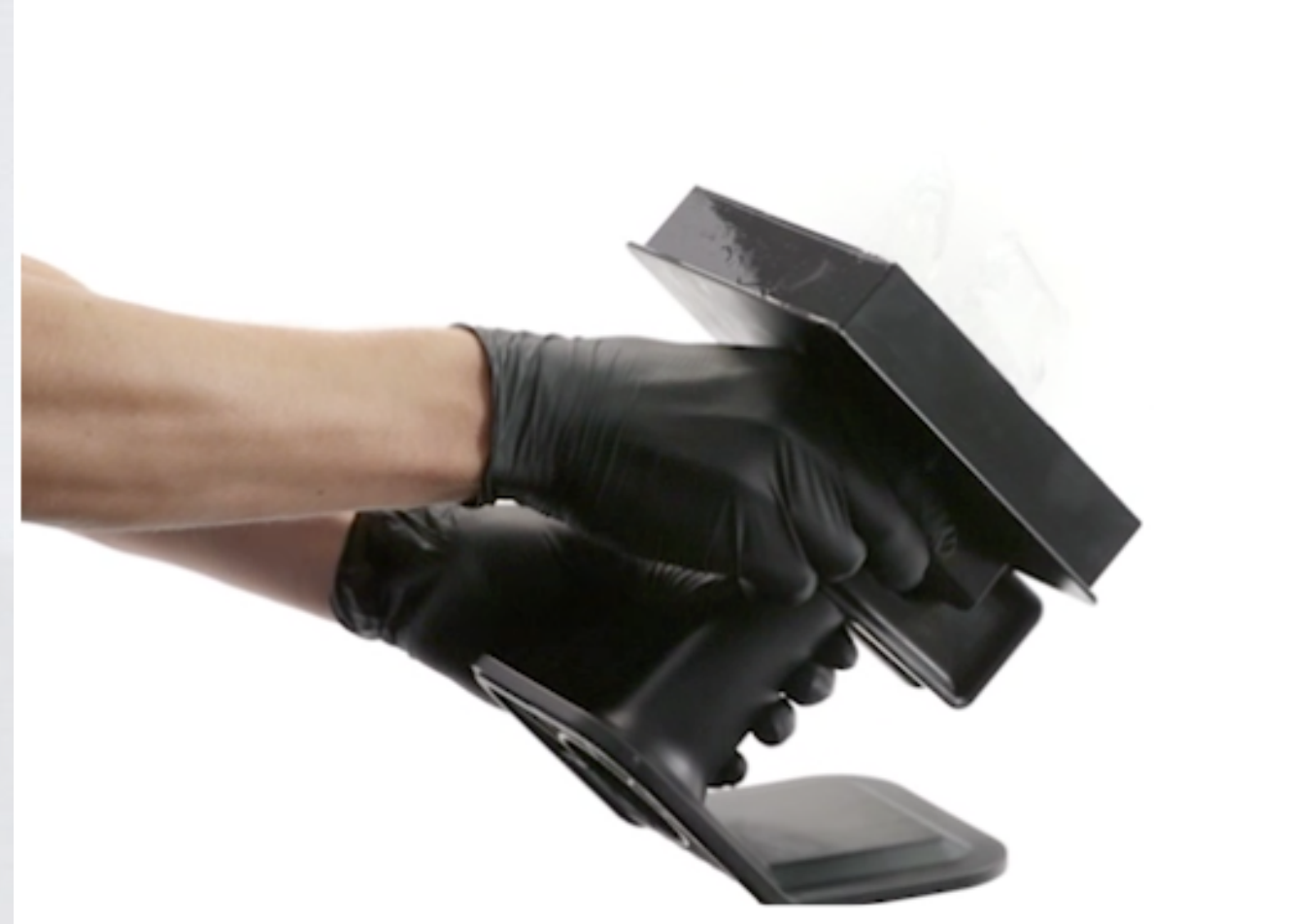
2. Put the build platform on the jig
