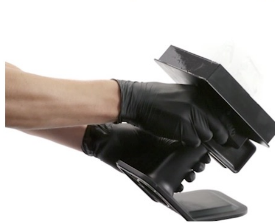
2. Put the build platform on the jig
